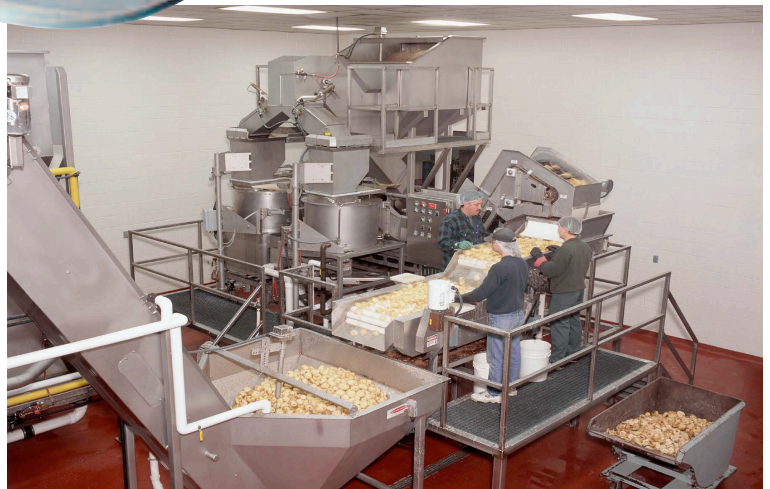
Custom systems are available with two-stage batch peelers, dewatering hoppers, diverting chutes, inspection/trim conveyors and platforms.
